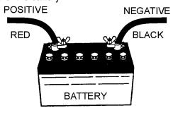
Figure 10. Battery Connections
